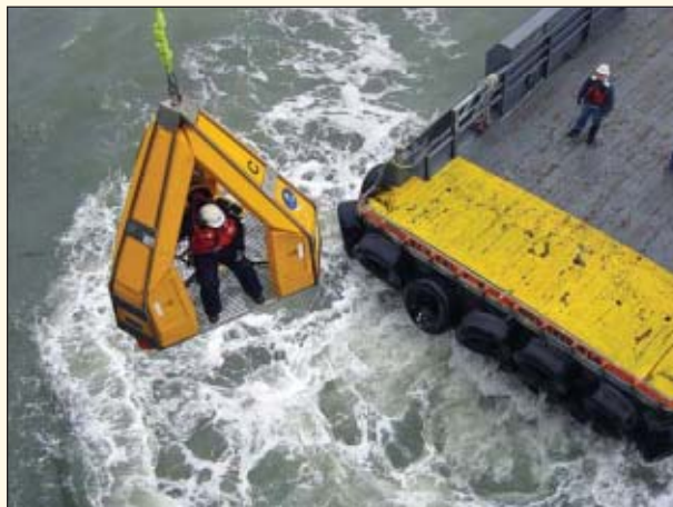
Reflex Marine Ltd., Aberdeen, developed a transfer capsule called the Frog in which riders strap into seats inside a rigid frame. Photo from Reflex Marine.
